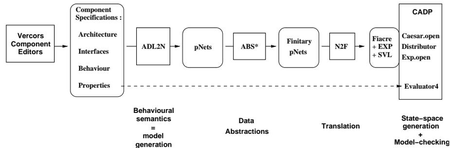
Figure 11: Tool chain and corresponding processing steps
