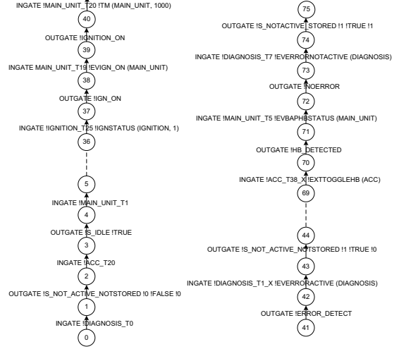
Figure 7. Test Case Covering Transition T7
